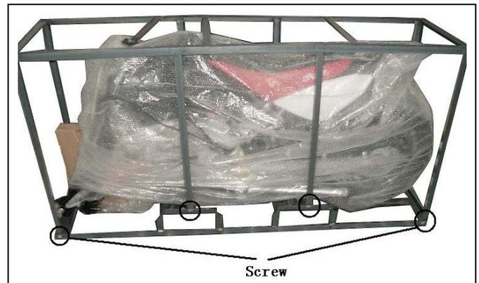
Remove the front axle bolt (17mm) and the shock absorber bolt (15mm) that are used to fasten the motorcycle to the metal cage. They are circled in the photo to the right. Pay special attention to the washers and bearings. Please refer to the diagrams in the service section if you are not sure how to re-assemble each bolt.
