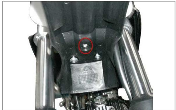
The number plate tab should be inserted just like the photo to the right. Securely tighten the three fender bolts. Next, fold the number plate upward and secure it to the upper triple clamp using the Phillips head screw circled in the photo to the right.
